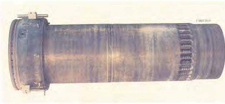
(H) Bore cooled RTA cylinder liner (Sulzer)
