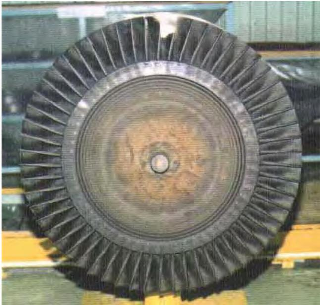
Fig. 98 Fatigue crack in turbine blade (Author)
