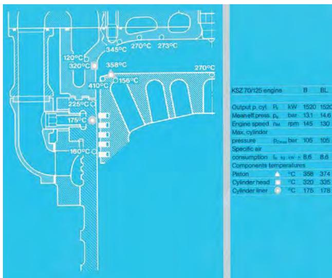
Fig. 66 Comparison of combustion chamber temperatures between K SZ70/125B and K SZ70/125BL. (MAN)
