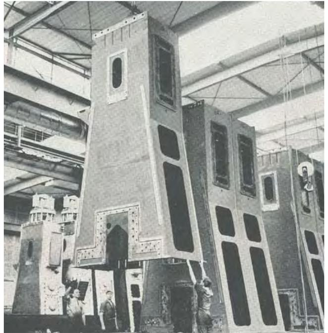
Fig. 53 Engine columns ready for assembly. (GV [3])
