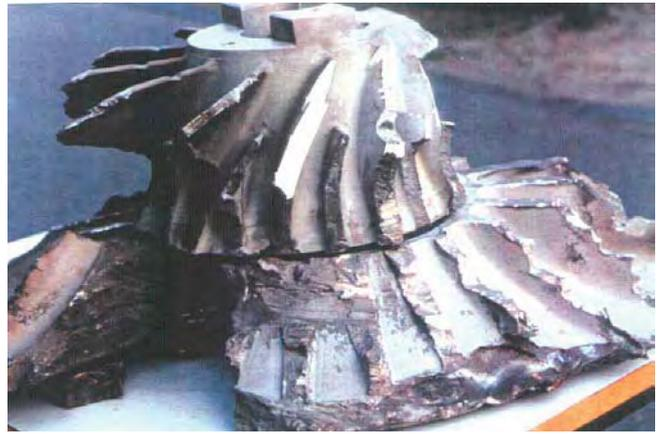
Fig. 99 Blower wheel of complete wrecked turbocharger (Author)
