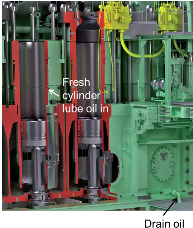
Figure 29 Scavenge drain oil
