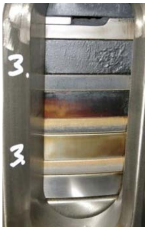
Same engine as opposite picture. Port inspection, cyl. 3. 1687 running h. Cylinder lube oil: 70 BN, low feed rate, ACC=0.26. Note: The cylinder lube feed rate is too low -> high wear and dirty ringlands
